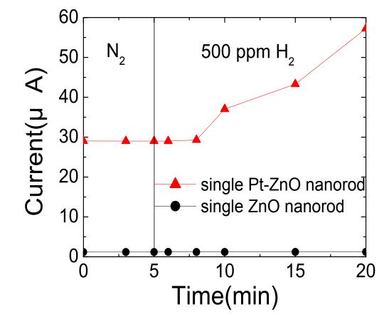
500ppm  $H_2$  test by with and without Pt-coated single nanorod (V=0.5V).
